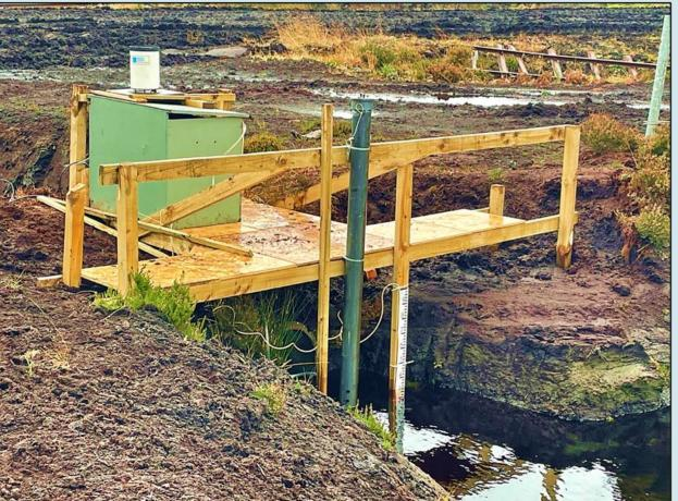
velocity flow meter and a Teledyne ISCO Sampler. The Sonde and flow meter were then moved to another station at the inlet. This, in addition to grab sampling, allowed the performance of the pond to be evaluated. The ISCO Sampler monitored during storm events. The monitoring included measurements of temperature, pH, electrical conductivity, turbidity and nutrient concentrations.
